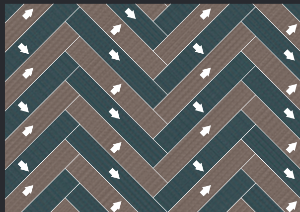
Two-colour herringbone pattern with warp weave planks and weft weave planks.
